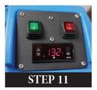
After plugging in all the heating elements and ensuring all the lights are lit, turn on the fan (GREEN SWITCH), then turn on the heater (RED SWITCH).
